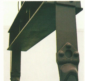
The Springplate upper pitman connection has no moving parts to replace.
